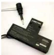
the BID will send a signal to the charger that the electrolyte level is low, and the control will display a message instructing the operator to check the battery.
