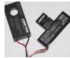
When equipped, a battery with an ampere-hour accumulator BID will transmit to the EC2000 control, the updated AH data.
