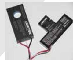
When equipped, a battery with an ampere-hour accumulator BID will transmit to the EC2000 control, the updated AH data. The accumulated AHs
