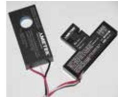
When equipped, a battery with an ampere-hour accumulator BID will transmit to the EC2000 control, the updated AH data. The accumulated AHs for both charge and discharge cycles are stored in the BID along with the lifetime average battery temperature, and is readable from the EC2000 control and through the Datalink<sup>2</sup> System.
